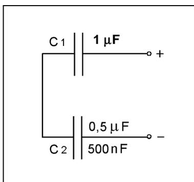
$$C_T = \frac{C_1 \times C_2}{C_1 + C_2} = \frac{1 \times 0,5}{1 + 0,5} = \frac{0,5}{1,5} = 0,33$$
