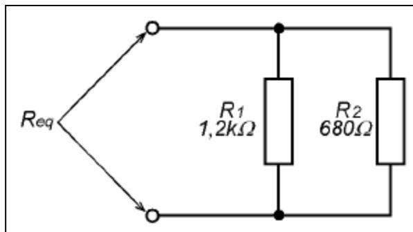
$$R_{eq} = \frac{R_1 \times R_2}{R_1 + R_2} = \frac{1200 \times 680}{1200 + 680} = \frac{816000}{1880} = 434\Omega$$
