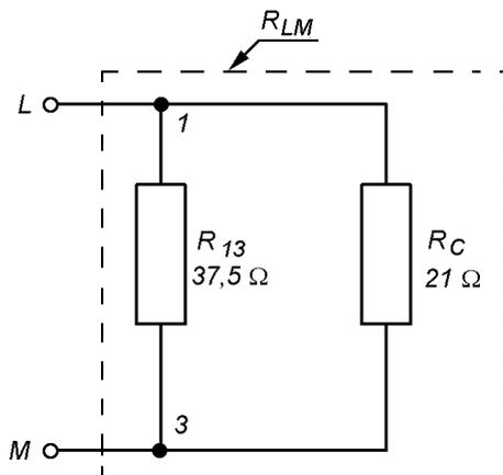
$$R_{LM} = \frac{R_{13} \cdot R_C}{R_{13} + R_C} = \frac{37,5 \cdot 21}{37,5 + 21} = \frac{787,5}{58,5} = 13,46 \Omega$$
