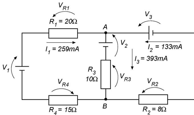
$$V_{R1} = R_1 \cdot I_1 = 20 \cdot 0,259 = \mathbf{5,18 \text{ V}}$$
